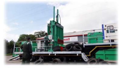
The MKII Baler remains mostly unchanged when compared with its static counterpart, but does benefit from additional floor structures to bolt to the trailer, and an easy to collapse head mechanism which reduces the overall height of the system to safely drive on the public roads without hitting bridaes.
