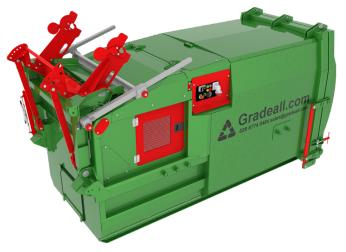
Manual loading doors are available on one or both sides of the GPC S9 if a bin lift is fitted.
